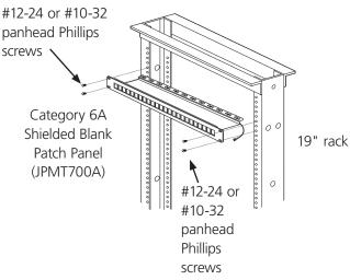
Figure 1. Panel installation.
